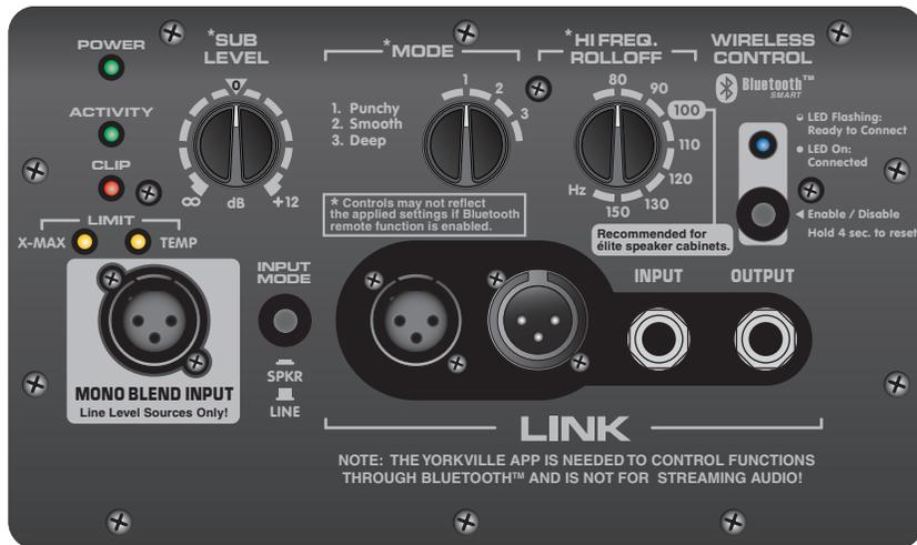
A '12 o'clock' setting on the ES Series Powered Subwoofer's Level control is the correct starting point when setting up a sound system. The '12 o'clock' mark refers to the setting that will give full power when the line input is used and the input signal is at a level of +4 dBV.
